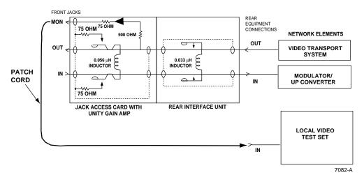
Figure 23. Non-Intrusive Video Test Access
